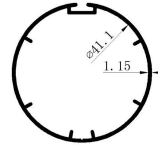
Item No.: GL1001 W: 0.473kg/m T: 1.5mm OD: \Phi 43.4mm ID: \Phi 41.1mm
